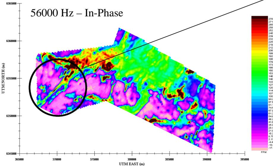
A linear, northeast trending anomaly in the southwest portion of Block 1 is visible across all frequencies (both in-phase and quadrature components). This is in the same area as the model for the magnetic data.
