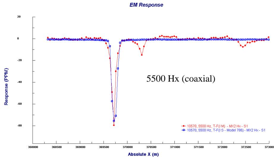
The plots compare the in-phase component of the data and Model 786 for 3 frequencies. (Line 10570)
