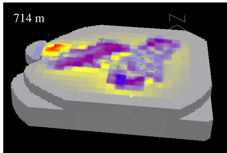
The magnetic data over Blocks 1 & 2 was inverted. The structure from the inversion result is mostly deeper than in the model. It is useful for showing the trends of linear magnetic features in the area.
