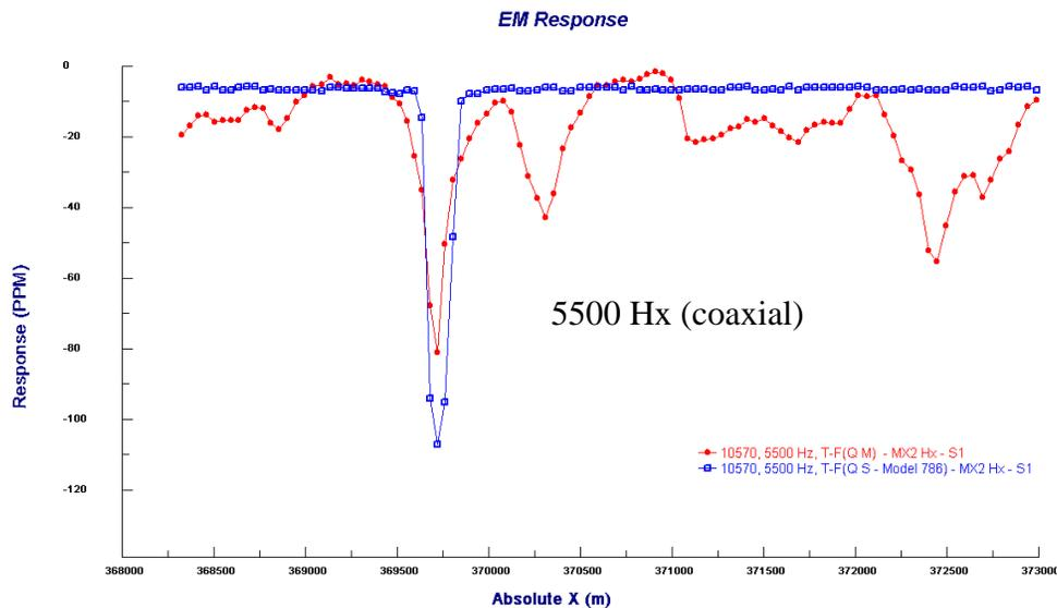
The plots compare the quadrature component of the data and Model 786 for 3 frequencies. (Line 10570)
