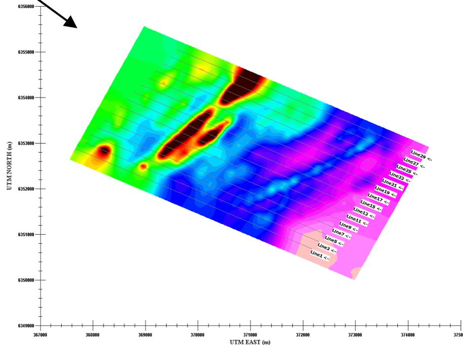
A section of airborne data in Block 1 where several linear anomalies are present was modeled. Derivatives were calculated for the gridded airborne data, and the gridded data with the derivatives was exported to profiles for modeling. \*Note that the data was exported to new lines, numbered 1-29. Lines 1-29 in the new profiles approximately correspond to Lines 10650-10490.
