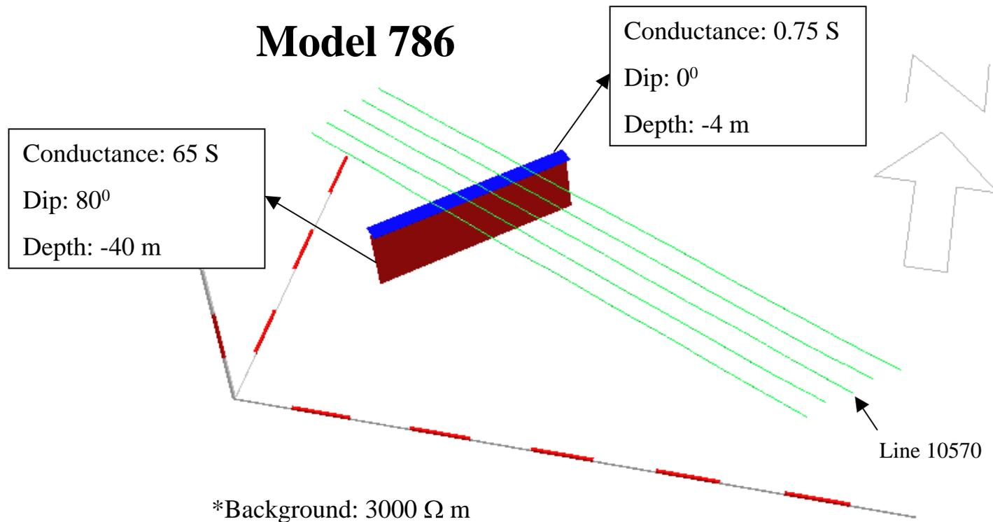
Plate models were used to investigate the induction response. Model 786 was developed to fit the EM data in the same area where the magnetic data was modeled. Two targets were needed to model the largest anomaly seen along these lines (to get both the in-phase and quadrature components to fit). These structures are slightly to the right of the structure in the mag model, but have the same strike.
