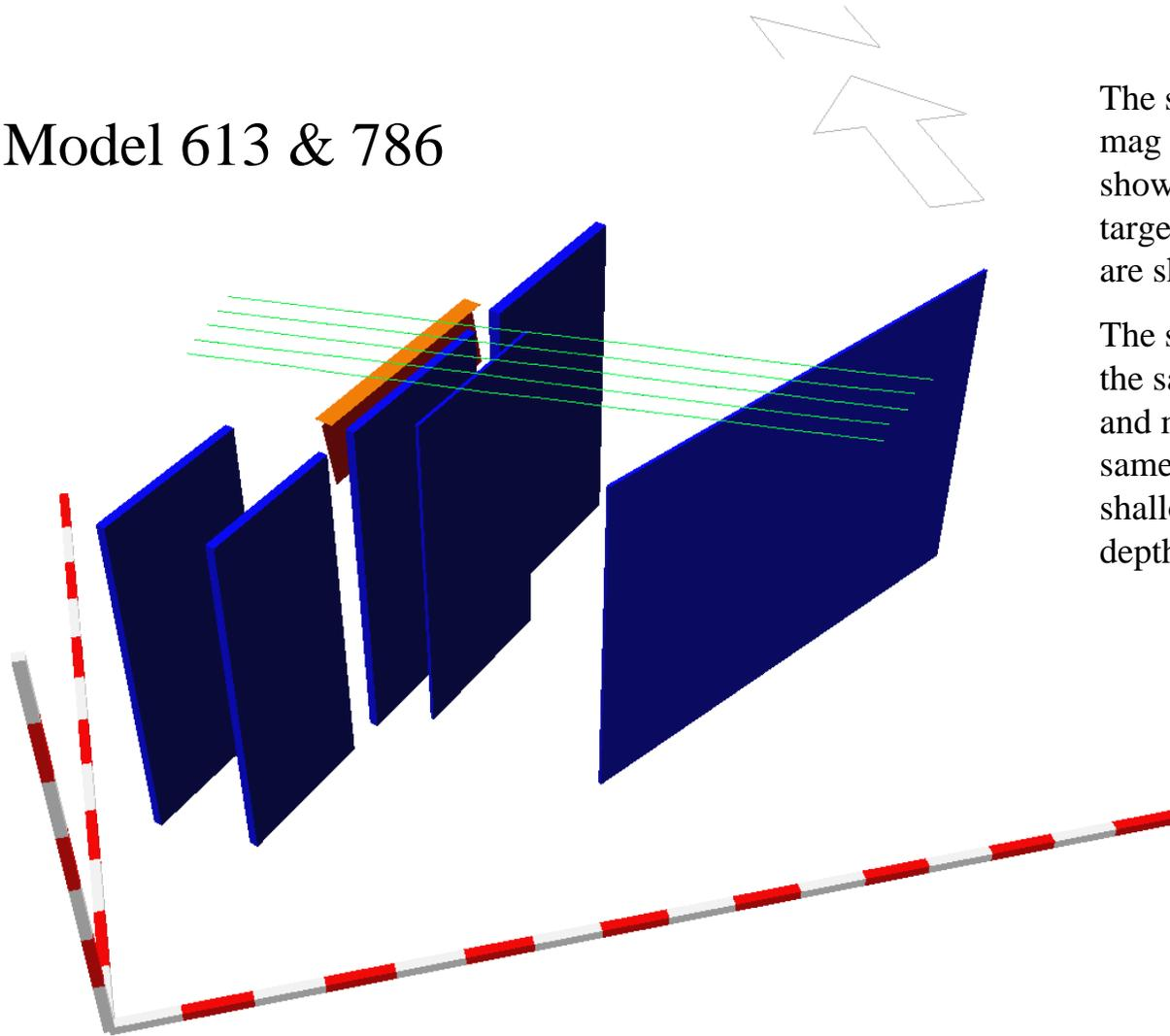
The susceptible targets from the mag model (Model 613) are shown in blue. The conductive targets from the EM model (786) are shown in red and orange.
